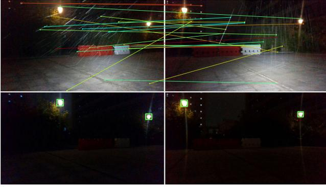
Fig. 2: Top row: active lighting results in a significant number of erroneous feature matches (colored dots and lines). Bottom row: object-level detection of streetlights (green detection boxes) remains extraordinarily robust even in completely dark nighttime scenarios.
