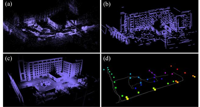
Fig. 4: Different map representations for vision-aided state estimation. (a) Visual feature point map. (b) Line map. (c) Point cloud map. (d) Streetlight map where the colored blocks represent streetlight instances and the gray ones are prior poses from the mapping process. Compared with (a), (b), and (c), (d) is a highly lightweight map containing both geometric and semantic object-level information.
